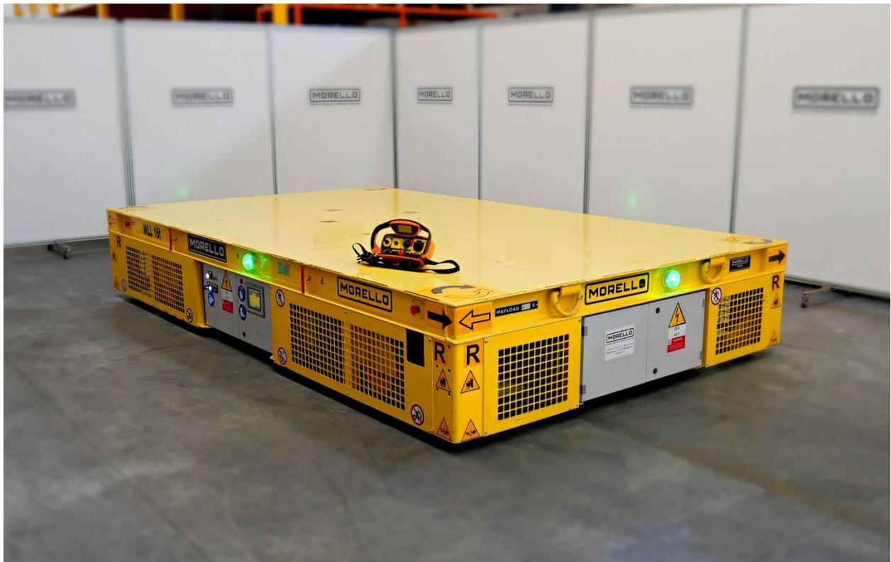
**SELF-MOVED ELECTRONIC OMNIDIRECTIONAL TRAILER, series SGAE-E OMNI-D R 16/2, operator on ground**, for factory material handling on concrete and asphalt flat and levelled floor
