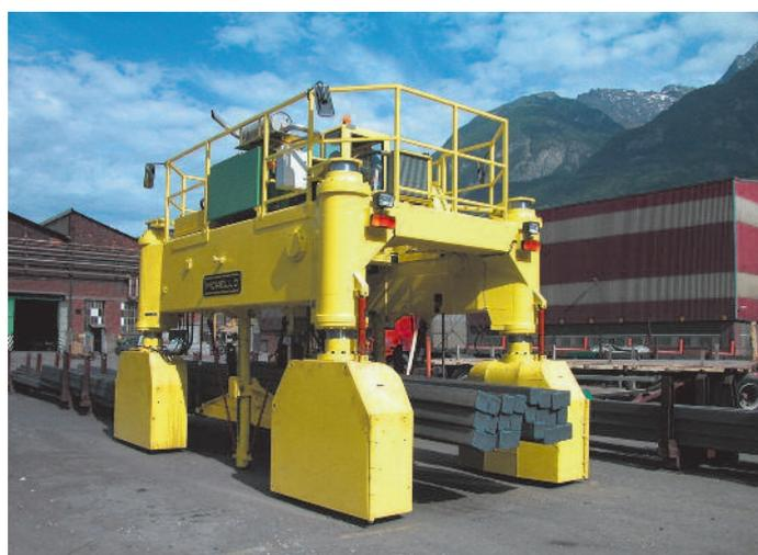
SEMOVENTI GOMMATI DIESEL PER CANTIERI NAVALI
